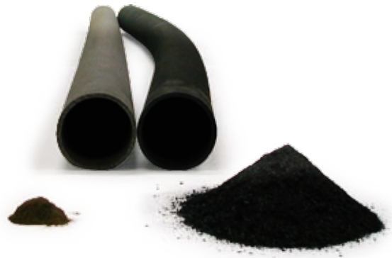
Fig. 4 Comparison of APMT Tube vs. Fe-35Ni-25Cr (after 2300 h at 2010°F). The FeNiCr tube is severely contaminated with oxide flakes.
